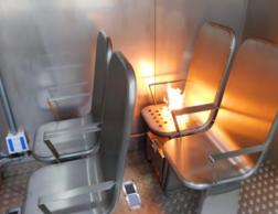
EDM's real fire trainer is designed and certified specifically to meet training requirements as defined in all international cabin crew training standards. It is designed for ease of operation from an instructional perspective with particular
